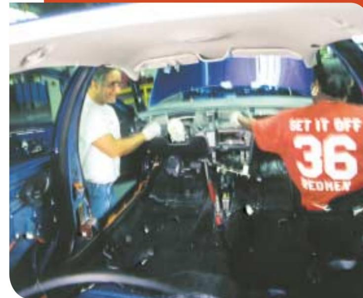
**MOVING AHEAD:** Above, Tom DiCintio and Michelle Colyar hook up the vent hose, route the heater control and set the dome light switch in place.
